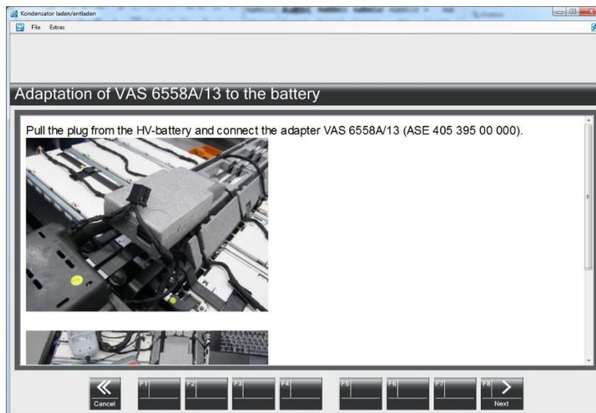
Fig. 4-20 Removing the plug from the HV-Battery
