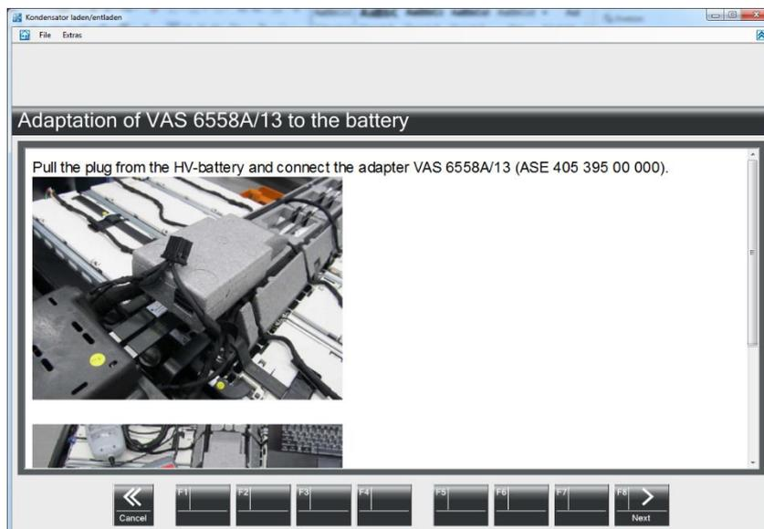
Fig. 4-37 Remove plug from the HV-Battery
